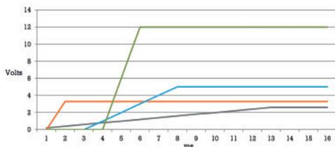
monitoring chips, to prove that the UUT will function as expected under the most extreme power-up cases. The diagram, to the left, shows an example of a complex power-up profile. This is easily achieved using two J-Testr supply peripheral cards, by adjusting the ramp rate of each individual supply, and the time sequence between each supply turning on.
