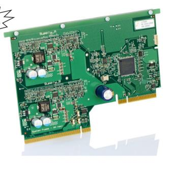
The supply peripheral card gives customers all the power supply features they would expect from a modern bench supply, all contained within the small footprint of a J-Testr peripheral card. In fact, with advanced features such as digitally programmable ramp rates, sequencing, and generic IO lines, these supplies offer capabilities only seen on more advanced expensive bench top supplies.
