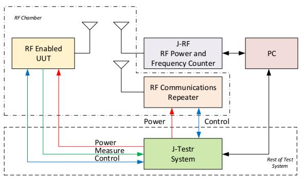
It is important that if such a 'repeater test' is implemented that the repeater device remains 'off' during the UUTs RF power and frequency measurement so it does not affect these sensitive measurements.
