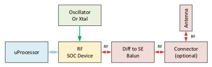
Figure 2 - Microprocessor, RF SOC and Balun Driven RF Power Path
