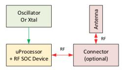
Figure 4 - RF SOC, with built in microprocessor, and direct driven RF Power Path
