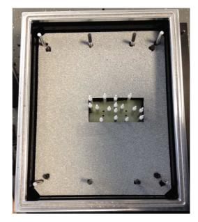
If production volumes require multiple test stations then it is extremely important that each test rig is a similar as possible within the RF chamber such that any reflected signal effects inside the chamber are consistent between different test stations. This is easily achieved with a good mechanical layout, the use of wireless receptacles (in test fixtures) and fixed sized ribbon cabling instead of individual wire wrap wires such as that shown below:
