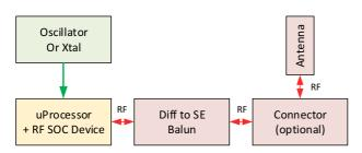
Figure 3 - RF SOC, with built in microprocessor, and Balun driven RF Power Path
