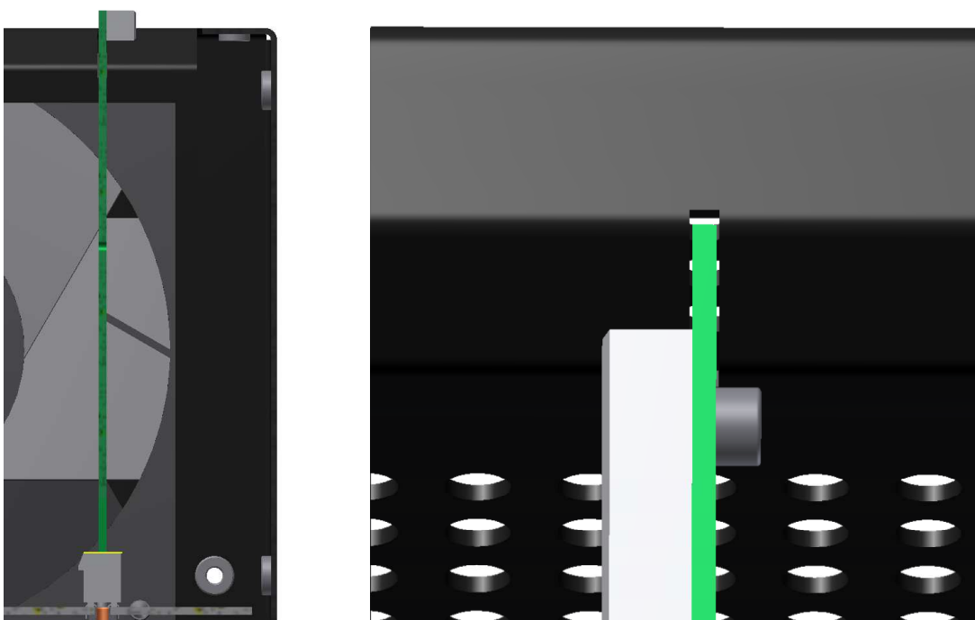
Figure 4 - Peripheral Card vertical insertion with mounting tabs aligned to tab location slots.
